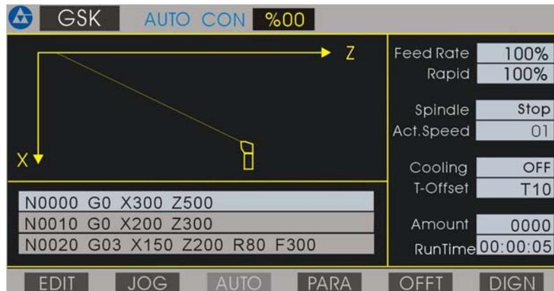
Fig. 19 Path of tool nose display in AUTO mode
