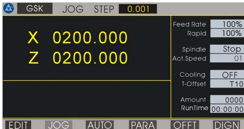
Fig. 12 Manual step feed mode
